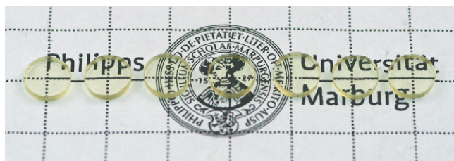
Fig. 3. Round polymer blanks of 5-FU-loaded HEMA/MMA polymer.
